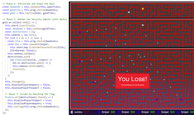
Figure 3: Code for an example challenge, Heist, that demonstrates the challenge creation API. Heist has three phases: (1) solve a maze to find the gold, (2) defeat the adversaries that appear when collecting it, and (3) solve another maze to escape. Players don’t know about these phases initially and are tasked with completing the challenge in the fewest attempts possible.
